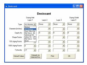
The program contains isotherms and property data for all the typical desiccants; activated alumina, 3A, 4A and 13X molecular sieve, granular silica gel, and spherical silica gel. Any desiccant diameter can be specified. Aging factors can be specified to study the impact of desiccant aging and contamination on dryer performance.
